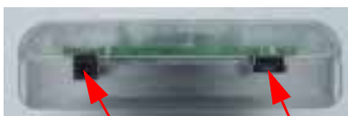
Low Voltage Connection Point (do NOT use)
