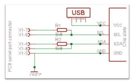
This simple scheme. In order to secure the CRUM and port, we recommend the scheme to the protection of the chip SN74LS05DR. That the scheme for the LPT port. For the programmer is required +5 V supply voltage. We recommend you take it from the USB connector on your computer.
