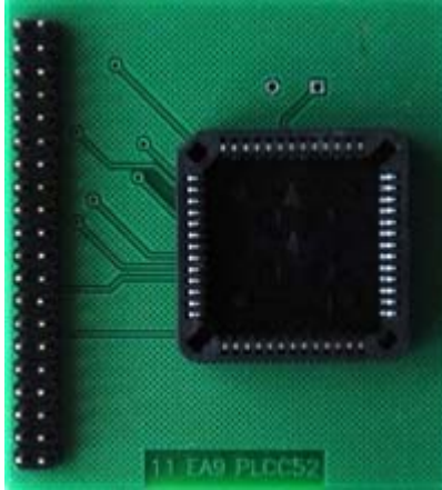
Figure 17. 11 EA PLCC-52 programming adapter
