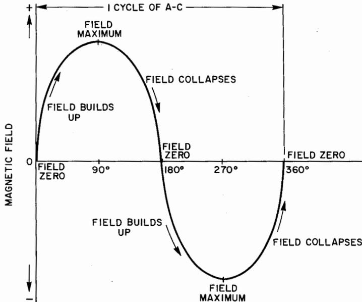
Fig. 24. Changes in the magnetic field from an alternating current.
