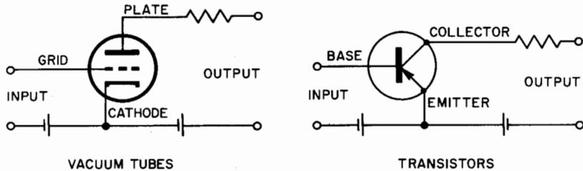
Fig. 65. Adjustable current devices.
