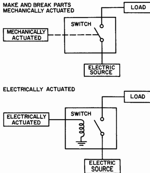
Fig. 70A. Make and break parts mechanically actuated.
