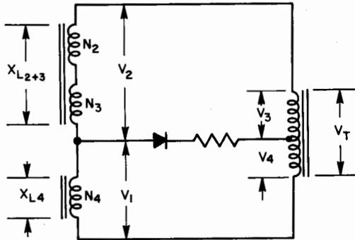
Fig. 53. Schematic diagram of a compensated magnetic amplifier.
