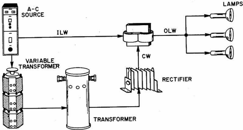
Fig. 80. Light dimming control system.
