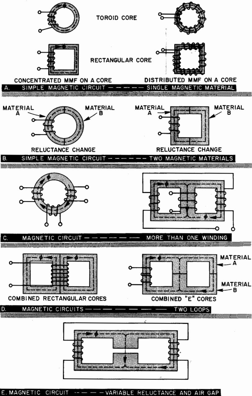
Fig. 28. Types of magnetic circuits.
