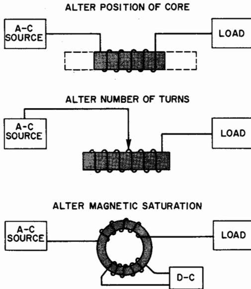
Fig. 69. Variable reactance methods.
