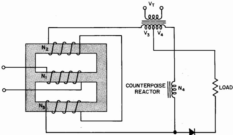
Fig. 51. Compensated magnetic amplifier.
