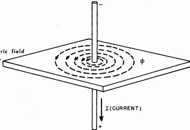
To determine the direction of a magnetic field around a conductor, grasp the conductor with the left hand, pointing the thumb in the direction of current flow. The fingers will then point in the direction of the magnetic field.
