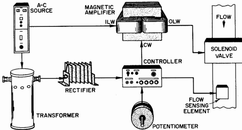
Fig. 79. Control of solenoid actuator valves.
