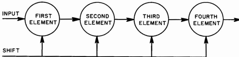
Fig. 99. Cascaded cores function as a storage register.
