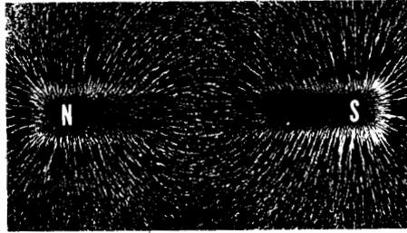
field is often referred to as *lines of flux*, or simply *flux*. They are often designated by the symbol " $\phi$ ". The unit of flux is one line and is called the *maxwell*. The flux per unit area, or the number of maxwells, is known as the *flux density* and is designated "B". The unit of flux density, or one maxwell per square centimeter, is called *gauss*. Therefore, by definition:
