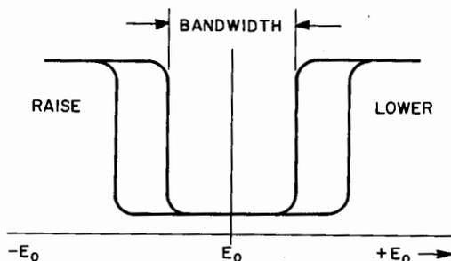
Fig. 93. Bistable output of a magnetic amplifier.
