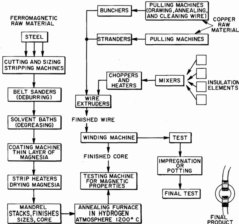
Fig. 74. Construction of a magnetic amplifier.
