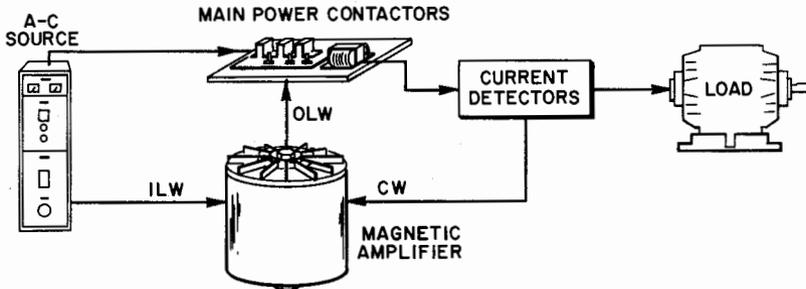
Fig. 81. Overload trip device.
