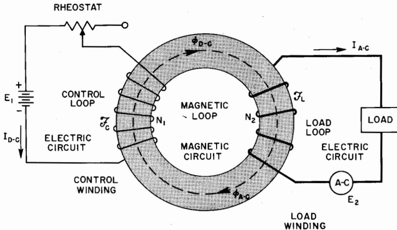
Fig. 30. Simple saturable reactor.
