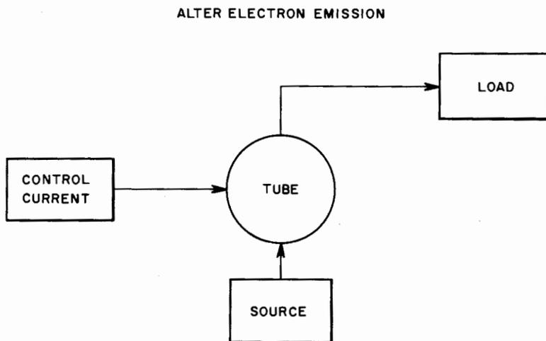
Fig. 68B. Variable thermionic emission method.
