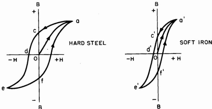
Fig. 22. Hysteresis loops for soft iron and steel.
