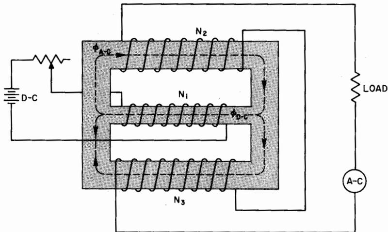
Fig. 47. Three-legged core arrangement to eliminate transformer action.
