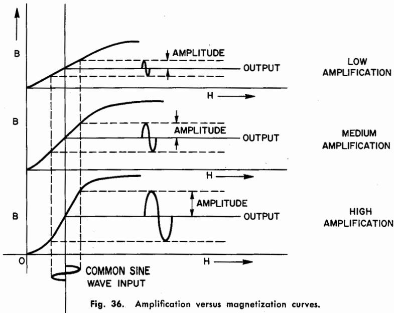
Fig. 36. Amplification versus magnetization curves.
