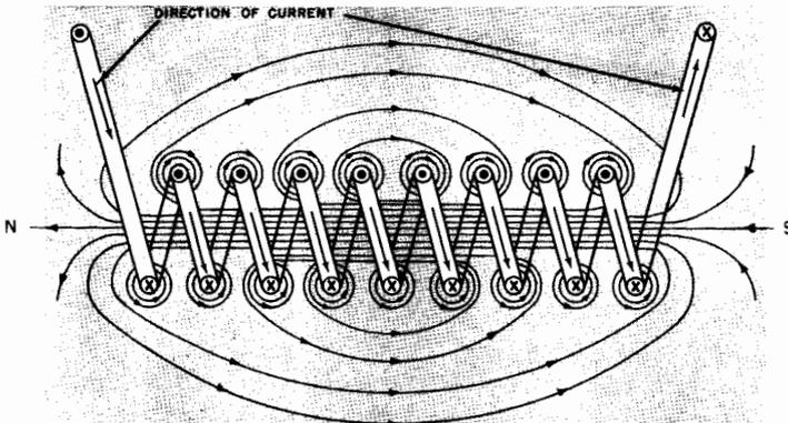
Fig. 16. Cross-sectional-view of a coil carrying a current.
