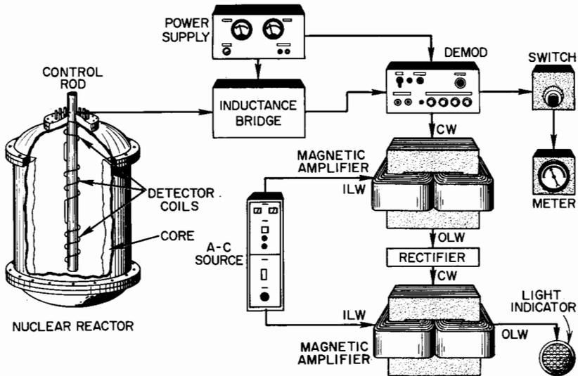
Fig. 96. Indicating system for position of control rod.
