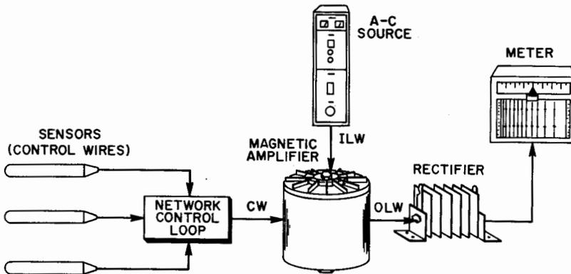
Fig. 86. D-c metering of large power lines.
