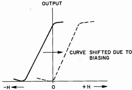
Fig. 55. Result of bias winding.
