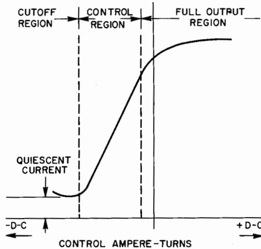
Fig. 42. Transfer characteristic of self-saturating magnetic amplifier.
