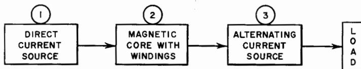
Fig. 29. Three essential elements of the saturable reactor.
