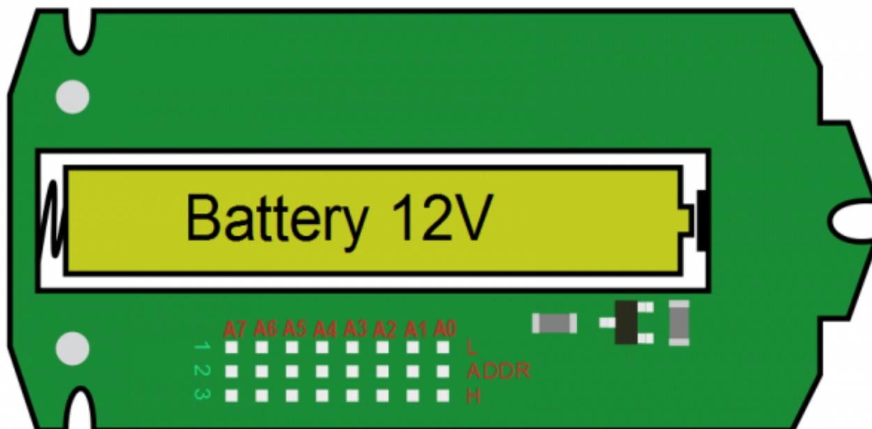
By three rows of metal welding points, the first row is grounding terminal, the second row is address pins,
