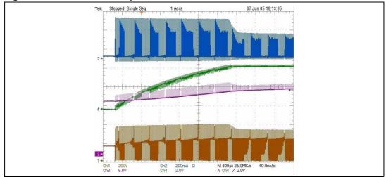
Figure 3. Full Load Start-up Waveforms at 115V
