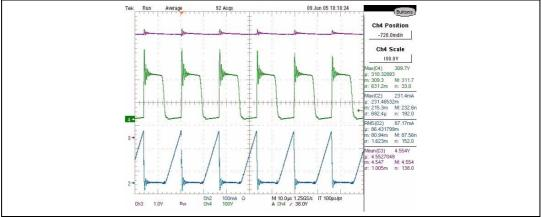
Notes: Magenta/Red (Ch3) = output voltage, Green (Ch4) = drain voltage, and Cyan/Blue (Ch2) = drain current.
