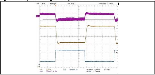
Figure 11. Step Load Change Stability Tests at 115V
