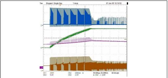
Figure 5. No Load Start-up Waveforms at 88V
