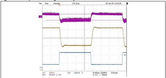
Figure 9. Step Load Change Stability Tests at 88V
