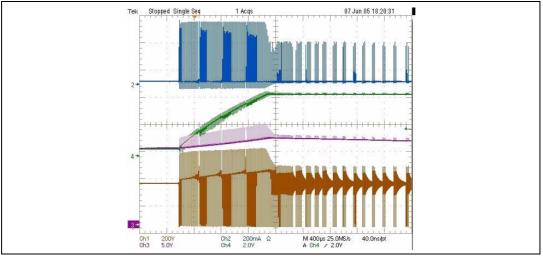
Notes: Cyan/Blue (Ch2) = drain current, Green (Ch4) = output voltage, Magenta/Red (Ch3) = auxiliary output voltage for the VIPer12A self-supply (on V<sub>DD</sub> pin), and Yellow (Ch1) = drain voltage.
