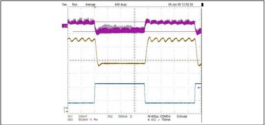
Notes: Magenta/Red (Ch3) = output voltage, Yellow (Ch1) = feedback pin voltage, and Cyan/Blue (Ch2) = output current.
