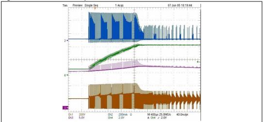
Figure 7. No Load Start-up Waveforms at 115V
