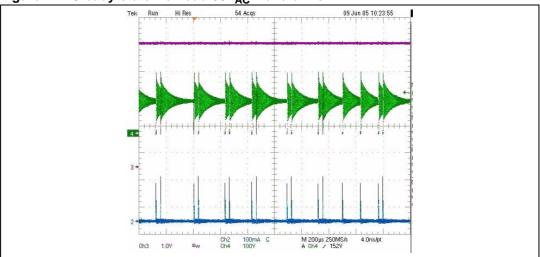
Figure 17. Steady-state No Load 88V<sub>AC</sub> Waveforms
