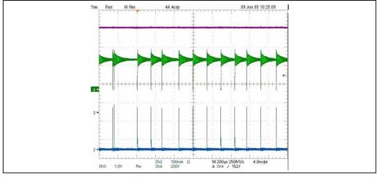
Notes: Magenta/Red (Ch3) = output voltage, Green (Ch4) = drain voltage, and Cyan/Blue (Ch2) = drain current.
