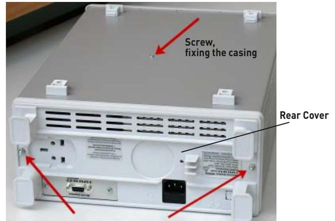
Figure 5-3: Back-Bottom View of HM5014-2 without handle
