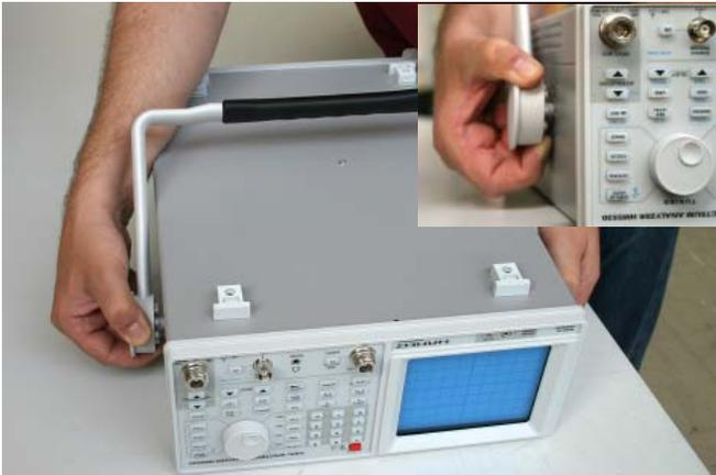
Figure 5-1: Removing Handle
