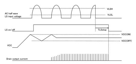
(C) Usual start and stop of LS detect SO signal mode (SO is connected to external parts)
