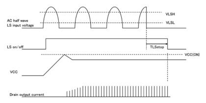
(B) Slow start and stop of LS start/stop mode (SO is connected to VDD)
