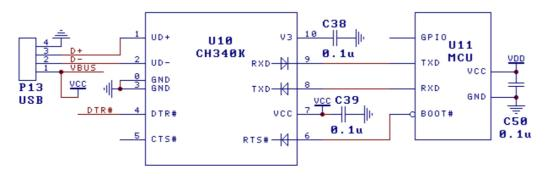
The figure above shows the reference circuit for USB communication between the MCU and the CH340K via UART. CH340K is powered by the USB bus VBUS (VCC), the MCU uses another power supply VDD, which supports 5V, 3.3V or even 2.5V, 1.8V. The backplane of the CH340K package is an optional GND pin that can be easily connected to GND or left floating depending on the PCB trace.
