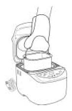
Mount the kneading blade on the shaft, flat side down.
