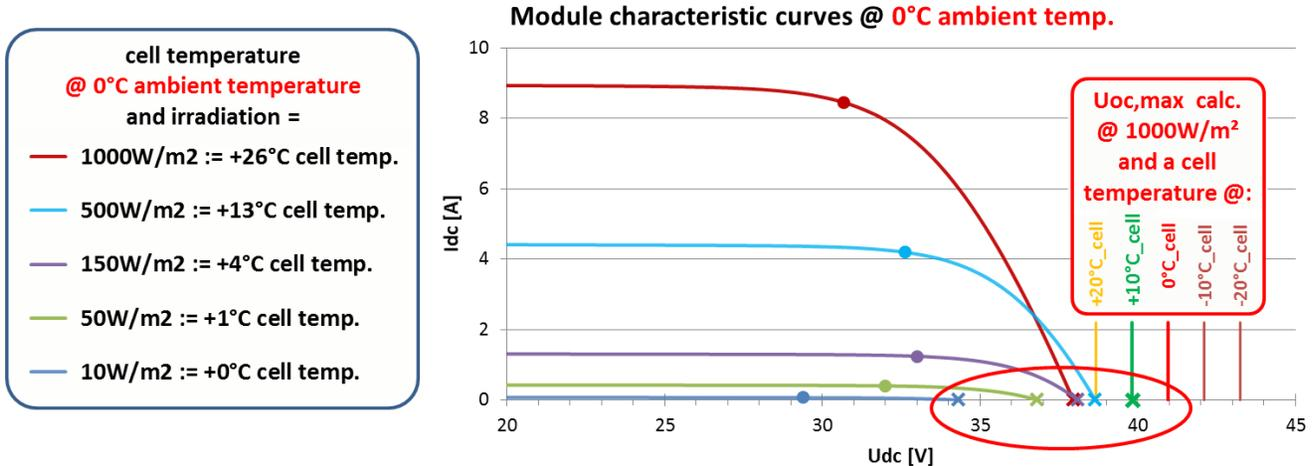
Table 1: resulting cell temperatures at an constant ambient temperature (0°C) at different irradiation levels.
