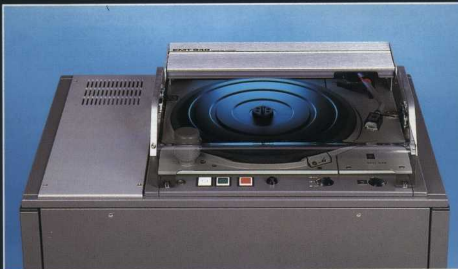
EMT 948 in console version with built-in cue amplifier, additional cartridge illumination, and simplified transport lock that is of particular advantage in mobile van use
