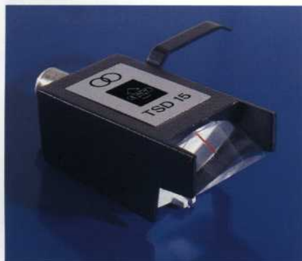
Dynamic cartridge with small effective mass at the stylus tip
