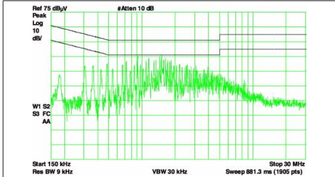
Figure 22. 115V<sub>AC</sub> Line Neutral
