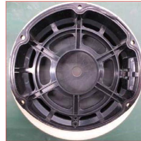
11. Use screwdriver 3.0 to remove 6pcs screws from left & right Passive Radiators.
