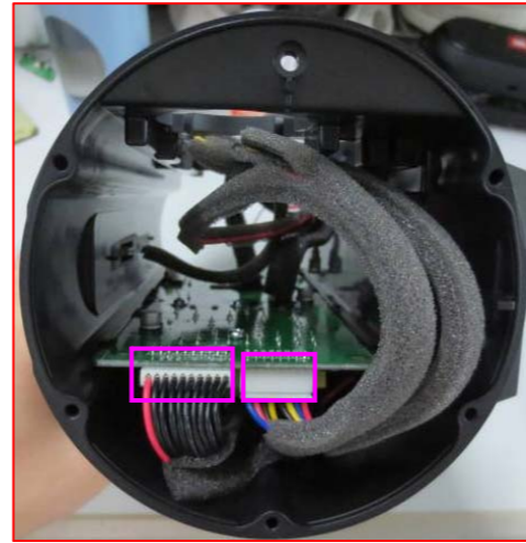
13. Pull out the speaker wire and connection wire on I/O board
