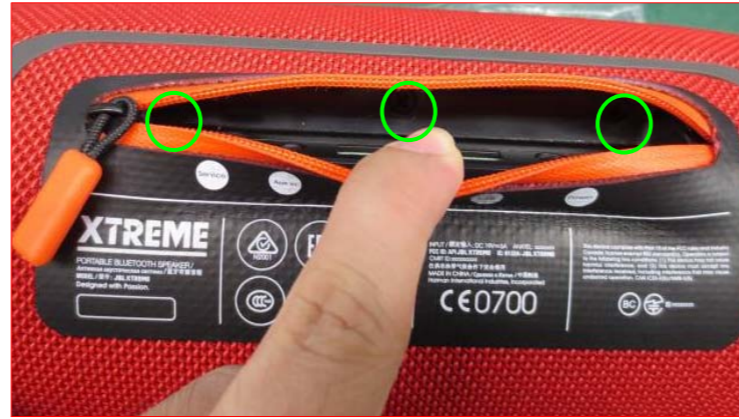
2. Use screwdriver 3.0 to remove 3pcs screws from bottom cover.
