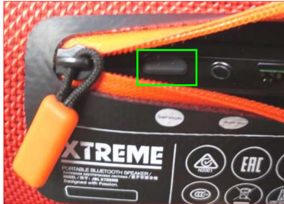
1. Unzip the set, pull out the rubber cover from Micro USB socket.
