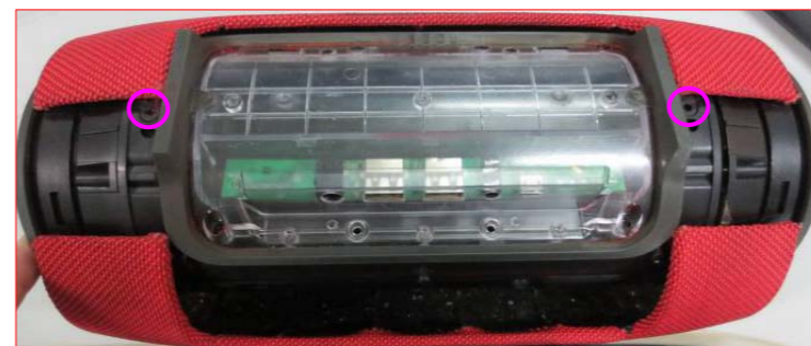
5. Remove 2pcs screws using screwdriver 3.0.
