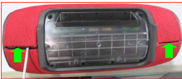
4. Use straight screwdriver to pry Grille off.
