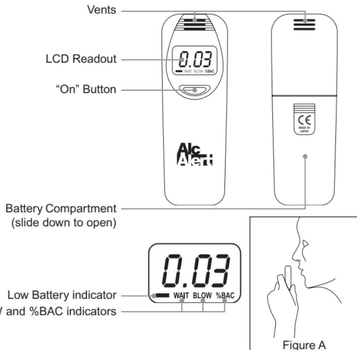
1. Press the “On” button. The unit beeps once, the “WAIT” indicator flashes, and the unit begins a “warm-up” countdown from 14-to-0 or 6-to-0 (see Additional Information). You must wait until the countdown is complete. Proceed with step 2 only when the unit beeps twice and the “BLOW” indicator flashes.
