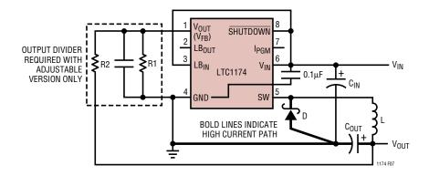
Figure 7. LTC1174 Layout Diagram (See Board Layout Checklist)
