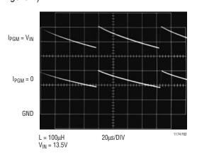
Figure 2. Inductor's Current with Output Shorted
