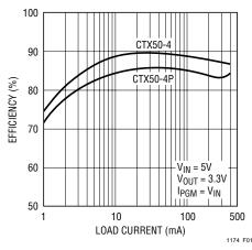
Figure 1. Efficiency Using Different Types of Inductor Core Material
