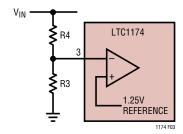
Figure 3. Low-Battery Comparator
