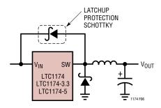
Figure 6. Preventing Absolute Maximum Ratings from Being Exceeded
