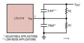
Figure 4. LTC1174 Adjustable Configuration
