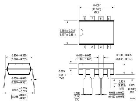
\*THESE DIMENSIONS DO NOT INCLUDE MOLD FLASH OR PROTRUSIONS. MOLD FLASH OR PROTRUSIONS SHALL NOT EXCEED 0.010 INCH (0.254mm)
