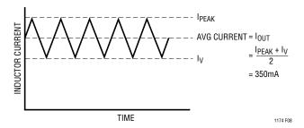
Figure 8. Continuous Inductor Current
