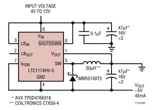
Figure 5. Positive-to-Negative 5V Converter
