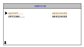
You can select Adjust or Options items by pressing Up/Down buttons. Selected parameter will be highlighted. Inorder to enter the selected parameter, press Left or Right button. To exit the service menu press MENU button. Entire service menu parameters of AK45 CHASSIS are listed below.
