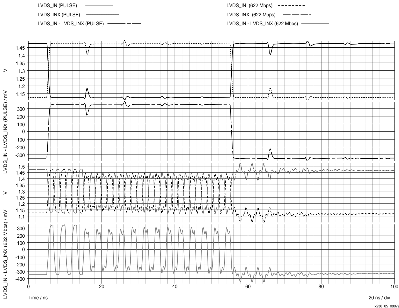
Figure 3: Typical LVDS Absolute and Difference Signals Showing Step and Burst Data Response at 622 Mb/s
