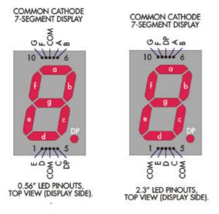
**LED Pinouts.** Pinouts are different for the two displays. See the top overlay of 3073A for the pinout details of each display. Note that two of the large 2.3" displays are mounted **upside down.**
