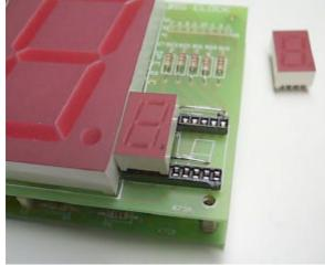
while the decimal points are driven via a 180R resistor. The 0.56" display segments are driven by 220R resistors.
