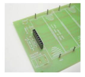
The three, **male** 8-pin connectors X4, X5 and X6 are to be soldered on the underside of 3073A so that, after soldering the two boards will fit together both mechanically and electrically. Note that the connectors
