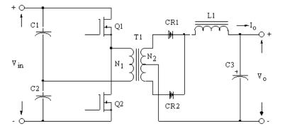
Figure 1. Half bridge converter
