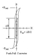
Figure 2 The dynamic BH loop of a push-pull converter.
