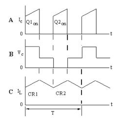
Figure 3. Typical half bridge converter waveforms.
