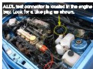
Locate the ALDL plug within your car. In this case it the 10-pin type can be found in the engine bay.
