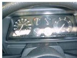
Get in the car and switch on the engine. The ECU light will begin to flash and pause a number of times. Take a note of the flash patterns.
