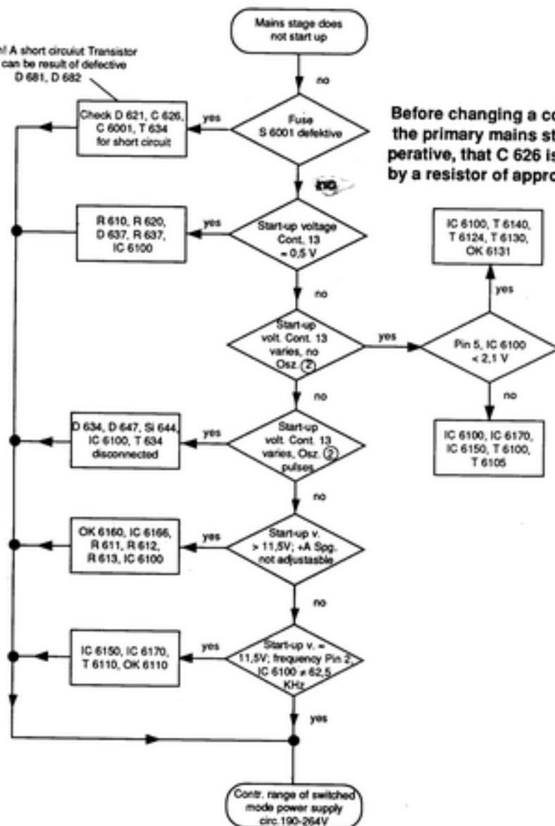
Before changing a component in the primary mains stage it is imperative, that C 626 is discharged by a resistor of approx. 100 Ohm.
