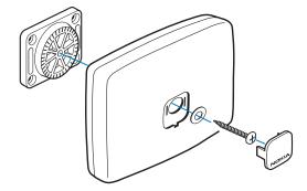
When installing the handsfree unit, ensure that the cables for the microphone and loudspeaker will reach the places you intend to mount these components.
