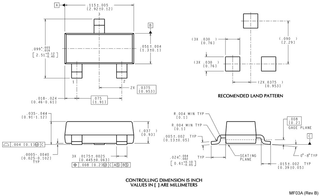
**SOT23-3 Molded Small Outline Transistor Package (M3)
