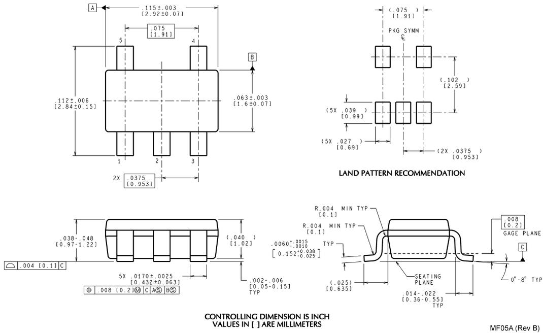
**SOT23-5 Molded Small Outline Transistor Package (M5)
