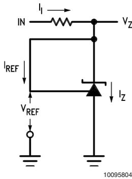
FIGURE 1. Test Circuit for  $V_Z = V_{REF}$
