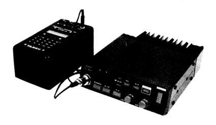
The FYG-4 is a microprocessor-controlled channel data programmer for the Yaesu FTL-2001 VHF and FTL-7002 UHF land mobile transceivers. Simplex and semi-duplex channel frequencies can be programmed, along with EIA standard RS-220-A subaudible CTCSS tones when the FTS-14 Tone Squelch Unit is installed in the transceiver.
