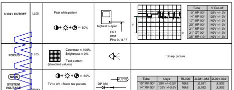
It is necessary to enter the Service Mode in order to carry out alignment of the TV set. Press the "Service" button on the RCU, except the "Focus" and "Volume" buttons.
