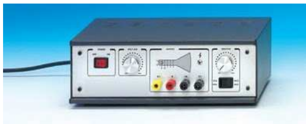
Figure 14: Photograph of a prototype of the regenerator CRT EN1659 in its case with anodized aluminum front and screenprinted. The article says clearly how to use this device, but in the absence of sufficient training in TV, get professional help (a television repairman).
