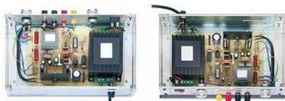
Figure 10: Photograph of a prototype of the regenerator plate CRT EN1659 installed in its case, to the back (top) and front view (bottom). These photos show what elements up front and the back panel, and they also show how to realize the interconnections between the plate and the two panels.
