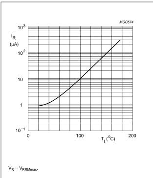
Fig.9 Reverse current as a function of junction temperature; maximum values.
