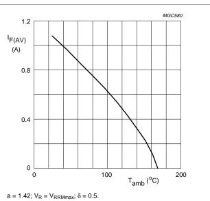
a = 1.42;  $v_R = v_{RRMmax}$ ; o = 0.5. Device mounted as shown in Fig.11. Switched mode application.
