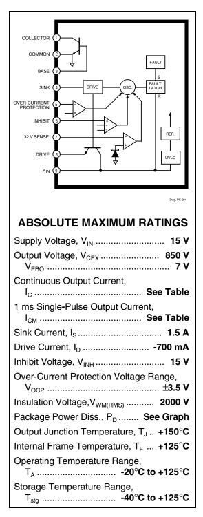
The STR-S5707 and STR-S5708 are specifically designed to meet the requirement for increased integration and reliability in off-line quasiresonant flyback converters with indirect feedback. Each device incorporates the primary control and proportional drive circuit with a third-generation high-voltage bipolar switching transistor.
