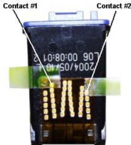
1. Put tape over Contact #1 as shown in the picture to the left. Place the cartridge back into the printer with the tape still stuck onto the cartridge.
