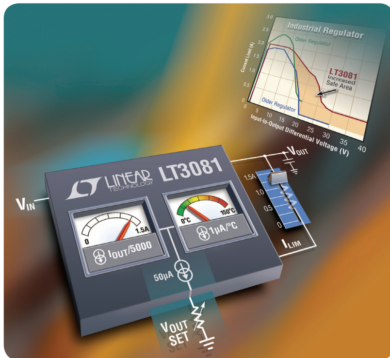
The LT3081 is one of a new breed of linear regulator, specifically featuring a wide safe operating area for industrial applications.
