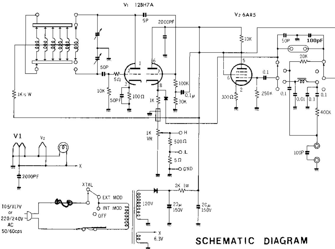
Addendum: Due to the low voltage used on B+, It has been noted that the 6AR5 is operating on the "knee" of a curve. Producing a distorted modulation pattern.
