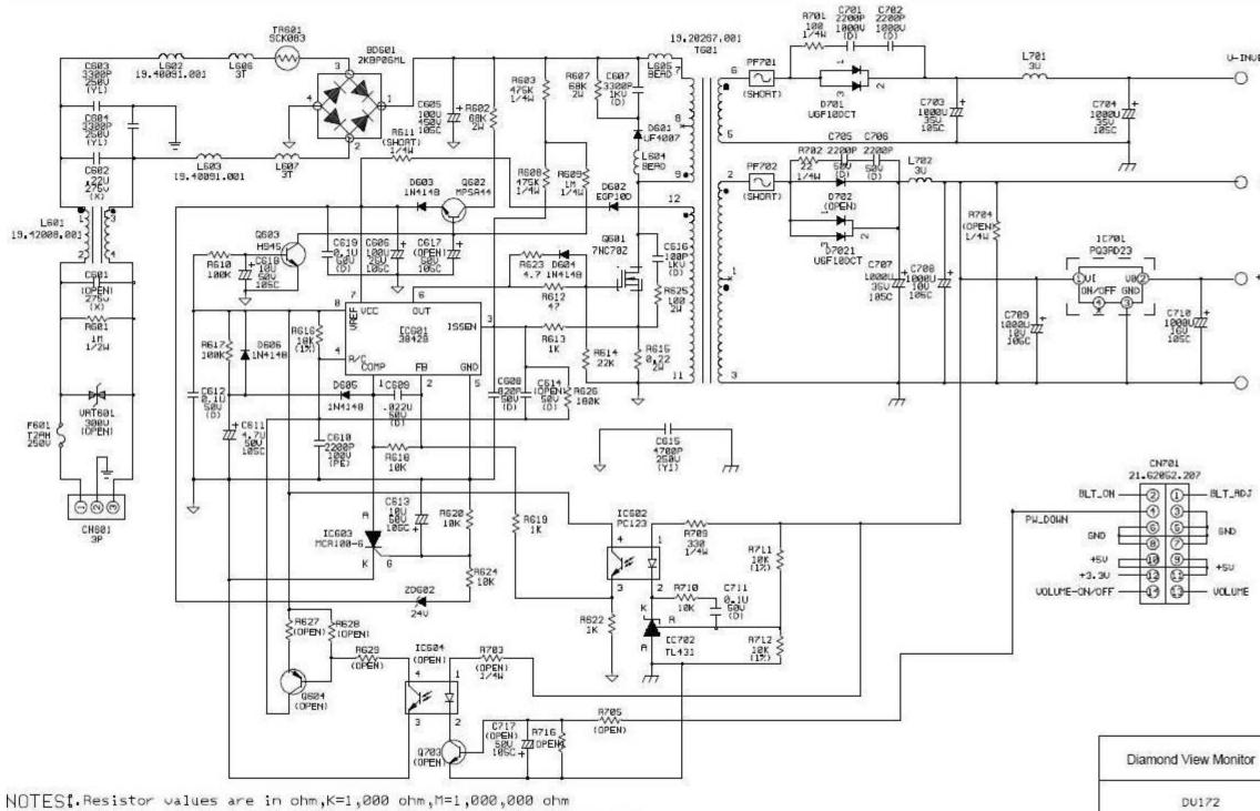
i believe that the following is the schematics for the benq inverter, i have not had time to check though
