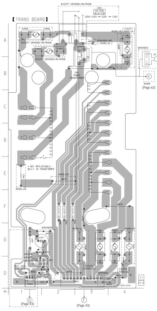
7-24. SCHEMATIC DIAGRAM - TRANS Board -
