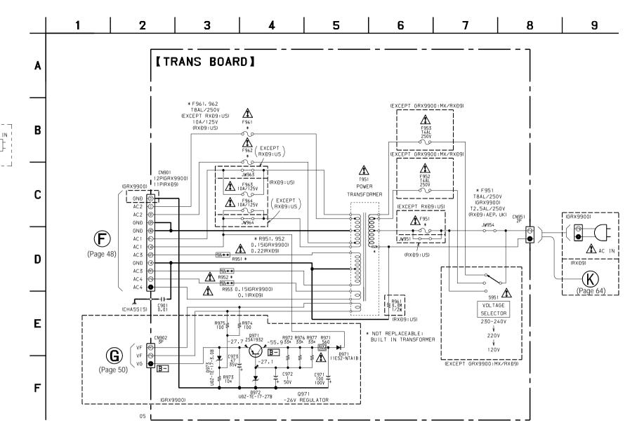
Voltages are dc with respect to ground under no-signal (detuned) conditions.
