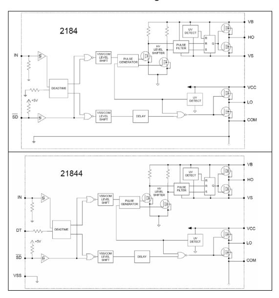
The IRS2184 and the IR2184 share the same block diagram. The IRS21844 and the IR21844 share the same block diagram. There are no functional changes between corresponding part numbers.
