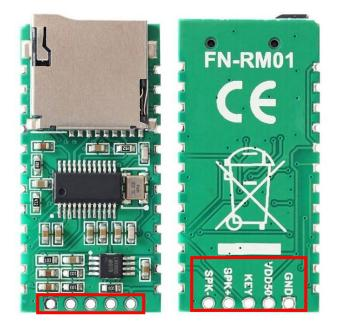
In order to connect to external buttons easily based on AD key control for users to accomplish button control, we made the solder pads at the bottom of the module as shown above marked with the red box. Through AD key function(the solder pad "KEY") and connecting with specific values of resistors, users can lead out 5 different functional key control as below. Please refer to the application circuits at page 19 for the connection in details of this part.
